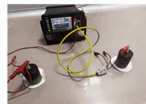
Surface resistance testing
