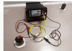
Leakage resistance testing
